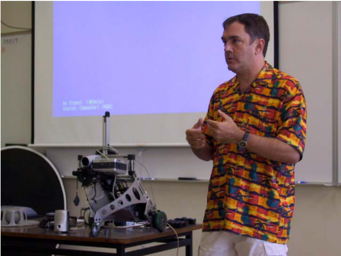
Steve Vorres gave a presentation on his Evolution 2 based robot with a video camera. This robot won the electrical outlet finding contest last month. He uses an actual video camcorder which provides better optics than most webcams and also has auto focus.
